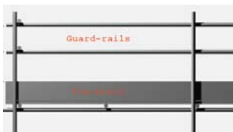
A guard rail with a mid rail and toe-board
